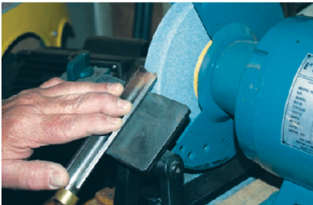
Better: create a more acute bevel angle on your tool, which will place it higher up on the wheel in a safer position when sharpening.
