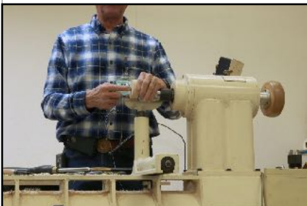
3. Drill 1/2" hole in center
