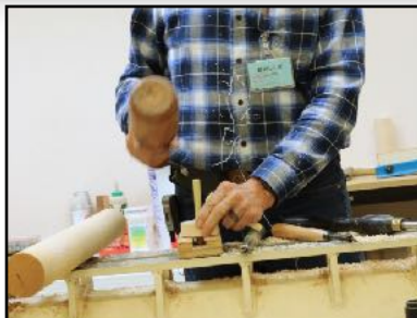
6. Drive dowel in hole 1/2" past disk for spinning tip
